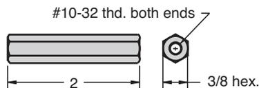
For providing space beneath assembled group of modules, use R-106 (order R-107-20, packet of four with hardware). Provides 2" clearance from enclosure wall for piping with Clippard fittings and tubing. Keeps piping and installation neat.
